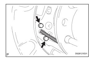
(b) Install the parking brake cable to the parking brake plate with the 2 bolts.
